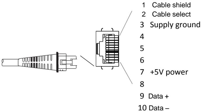
Note: Pin assignments are not compatible with legacy products. Use of a cable with improper pin assignments may lead to damage to the unit. Use of any cables not provided by the manufacturer may result in damage not covered by your warranty.
