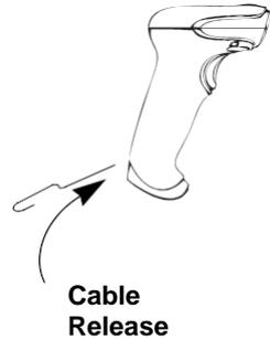
6. Replace with the new cable. Insert the connector into the opening and press firmly. The connector is keyed to go in only one way, and will click into place.
